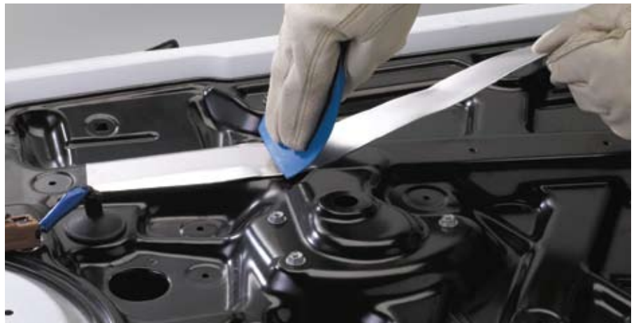
Applied with a 3M™ PA-1 Wiper to the inside of a car door, 3M™ Damping Foil 2552 effectively damps noise and vibration with as little as 10% surface coverage. Optimized acrylic on a dead soft aluminum constraining layer converts vibrational energy to negligible heat that readily dissipates.
