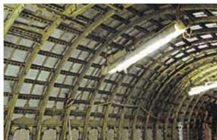
3M™ Damping Foil 435 between the ribs and stringers of an aircraft fuselage helps reduce vibrational fatigue and noise inside the passenger cabin.
