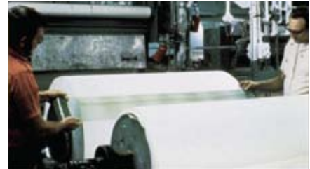
With thin caliper, high tensile strength polyester backing and the excellent shear strength of silicone adhesive, 3M™ Polyester Tape 8402 works well for butt splicing silicone-treated papers
