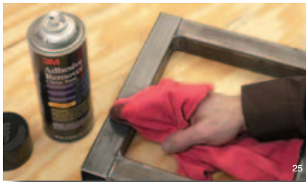
Spray 3M™ Adhesive Remover on metal parts and wipe away prior to adhesive bonding, tape application, painting, coating, or further processing. Removes soil and contaminants that could interfere with proper adhesion.
