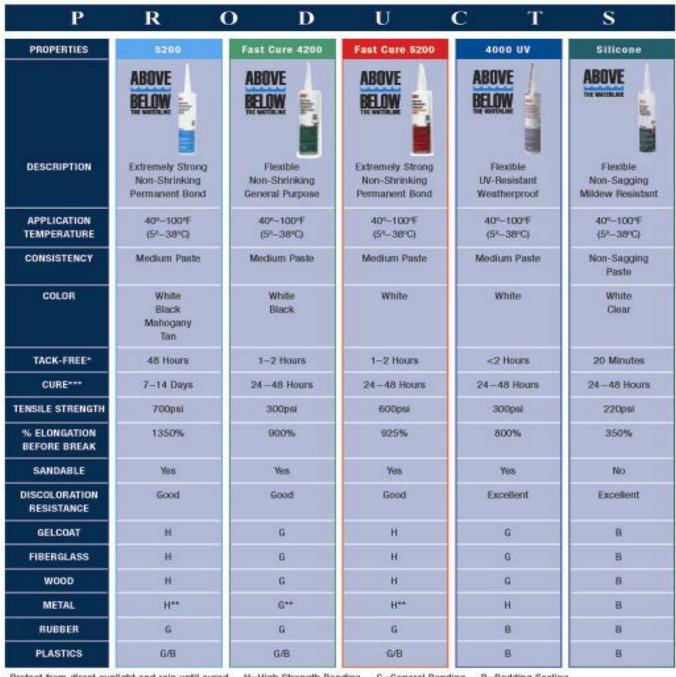
Protect from direct sunlight and rain until cured. H=High Strength Bonding G=General Bonding B=Bedding Sealing \*at 75°F/50% RH \*\*Primer recommended \*\*\*at 1/4° depth
